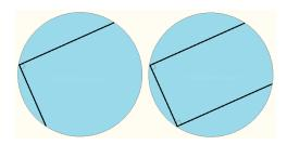
**Step 4:** Draw a line connecting the ends of the first and second chords. This line is the diameter of the circle.
