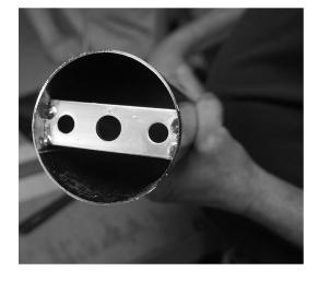
4. Flip over so spider plate faces the floor. Position base plate on column, rotating until it falls into place in the notch.
