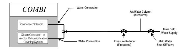
**Figure 2-10 Cleveland Range Single Water Supply Arrangement**
