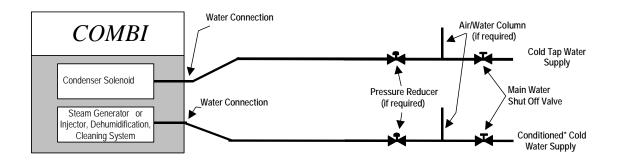
Figure 2-11 Cleveland Range Separate Water Supply Arrangement
