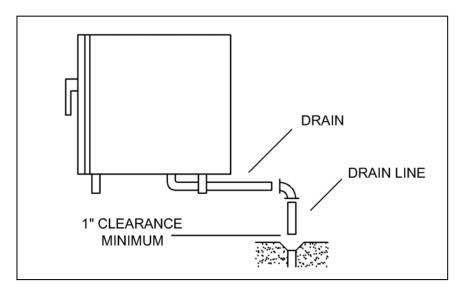
Figure 2-12 Typical Drain Layout
