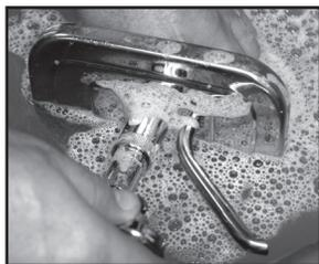
5. Wash and sanitize pump and components. Make sure to pump detergent and sanitizer through pump.
