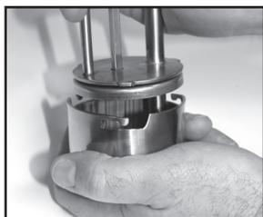
3. Remove bottom cap by twisting cap counter clockwise.
