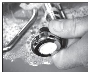
2. Wash outside of pump and immerse in wash water while pumping to clear any remaining food product.
