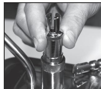
(Photo 2) Turn stem counter clockwise for a larger portion and clockwise for a smaller portion. Replace lever and set screw. Test the pump with the condiment to be dispensed and make additional adjustments if necessary.
